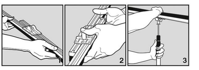
Extend the Span<sup>™</sup> and flip the red tab to lock it at the desired width. IMPORTANT: Notice the arrows on the red slide – the direction of extending the Span<sup>™</sup> is essential to its proper function.
