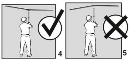
To seal a dust barrier at the ceiling, snap the Span™ onto the ball joint of a ZipWall® pole, raise the pole with the attached Span™ to the ceiling, and lock it into place.
