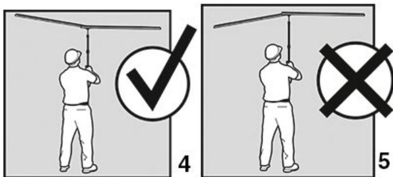
To seal a dust barrier at the ceiling, snap the adjustable tapeless seal onto the ball joint of a ZipWall® pole, raise the pole with the attached FoamRail™ to the ceiling, and lock it into place.
