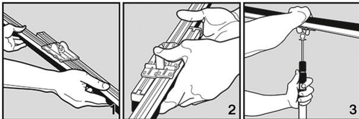
Extend the adjustable tapeless seal and flip the red tab to lock it at the desired width. **IMPORTANT:** Notice the arrows on the red slide – the direction of extending the tapeless seal is essential to its proper function (fig.4-5).
