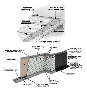
Inspect and Repair ... A thorough inspection should be made before covering and all necessary repairs made immediately. Tears and inadequate overlaps should be covered with MEL-ROL ... slit fish mouths and patch. Seal edges of all patches with POINTING MASTIC. Where applicable, horizontal applications can be floodtested for 24 hours. All leaks should be marked and repaired when membrane dries.
