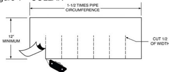
**Seal All Protrusions ...** Cut a slit around pipes, ductwork, rebar, and wire penetrations to place the initial layer of PERMINATOR. To further protect the concrete slab from external moisture sources, use a piece of PERMINATOR and place a collar around this as well.
