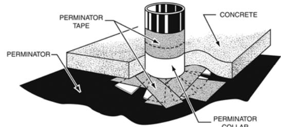
In the event that PERMINATOR is damaged during or after installation, repairs must be made. Cut a piece of the vapor barrier large enough to cover any damage by a minimum overlap of 6" (152.4 mm) in all directions. Clean all adhesion areas of dust, dirt and moisture. Tape down all edges using PERMINATOR TAPE.
