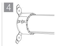
Fasten all collar anchor tabs to mounting surface using approved fasteners.
