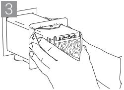
Insert Device into opening and install steel retaining plate and gasket on opposing side of wall. Secure plate to pathway by tightening hex head slotted screws. Ends of device to project equally from wall surfaces.
