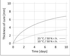
Diagram 1: Curing speed of Sikaflex®-511
