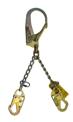
be used as a single-person positioning device on rebar forms, and features 2 double-locking snap hooks and a large swiveling rebar hook (designed to fit a Gates Form). Must be used for positioning
