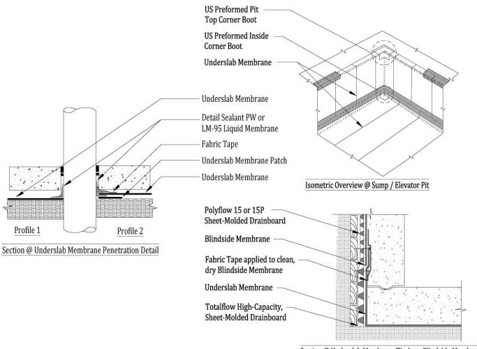
Section @ Underslab Membrane Tie-In to Blindside Membrane
