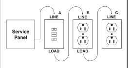
Placing the GFCI in position A will also provide protection to "load side" receptacles B and C. On the other hand, placing the GFCI in position C will not provide protection to receptacles A or B. Remember that receptacles A, B, and C can be in different rooms.
