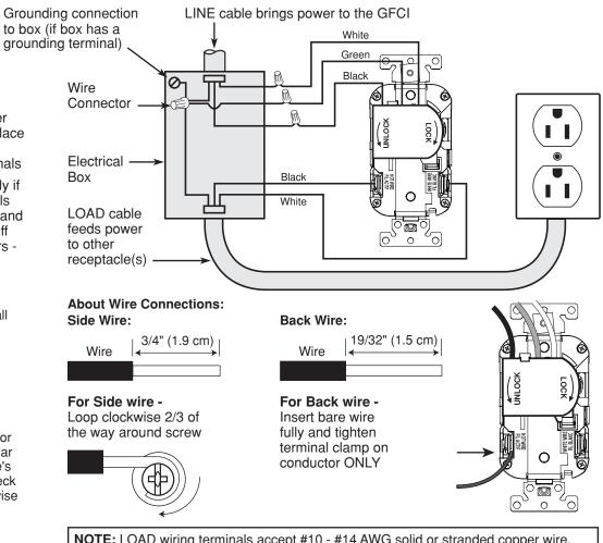
B: Two cables (4 or 6 wires) entering the box
