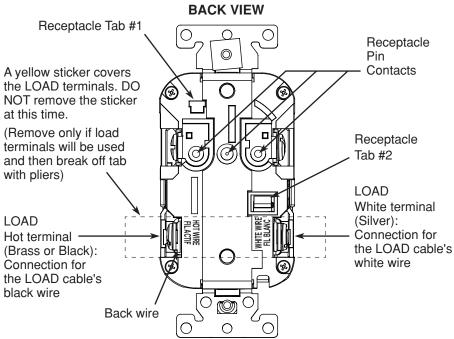
(a) Detach one cable's white wire and hot wires from the receptacle and cap each one separately with a wire connector. Make sure that they are from the same
