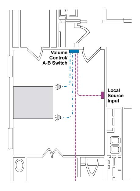
Four conductors of speaker wire and 1 CAT 5/5e
