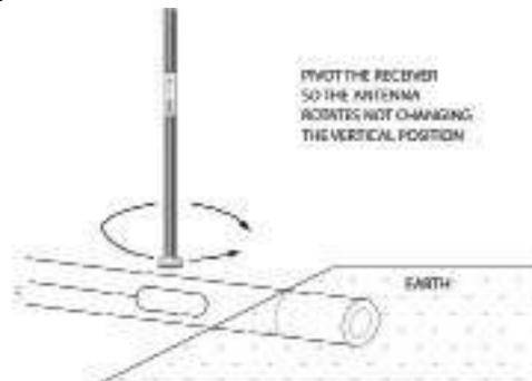
Now move Receiver side to side (across path of pipe) as shown below. When PEAK is found, Receiver is directly over Sonde. Mark this location. Next, check for ghost signals in front of and in back of Sonde to confirm location.
