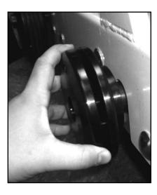
Figure 11: Separating the Flanges
