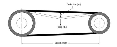
above when force (lb.) listed in chart above is applied to belt using
