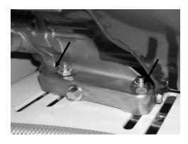
Figure 26: Engine without Adapter Plate/Mounts
