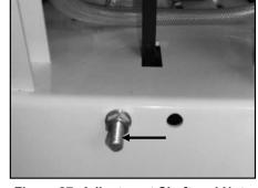
Figure 27: Adjustment Shaft and Nut
