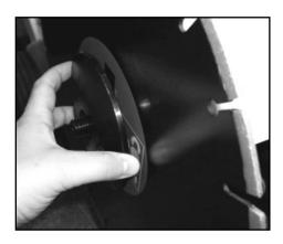
Figure 12: Inserting the Outer Flange
