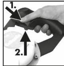
Always work with the ON/OFF switch fully pressed.
