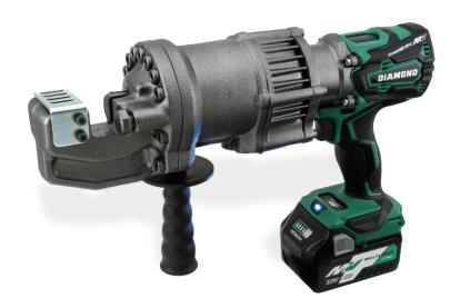
**The DCC-2036BHL cordless rebar cutter** will safely and cleanly cut rebar up to 3/4" diameter grade 60. This self-contained electric/hydraulic unit will also cut other items like chain, bolts, and rod. The DCC-2036BHL can be used in rescue operations. It can cut in close proximity to a trapped victim and does not throw sparks.
