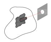
**4.** Cut a piece of DETAIL FABRIC to the dimensions of the soil nail plate and embed the fabric into the previously applied HYDRALASTIC 836.
