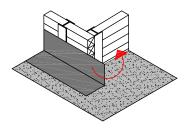
1. Install PRECON according to installation instructions onto soil stabilization system. Allow a minimum of 12" overlap to extend around outside corner.
