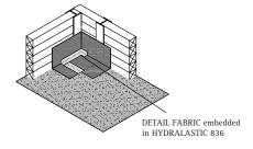
**5.** Apply HYDRALASTIC 836 at all overlapping joints in a 12" wide application and then fully embed DETAIL FABRIC into this HYDRALASTIC 836. Terminate all edges with additional HYDRALASTIC 836.
