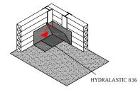
**4.** Apply HYDRALASTIC 836 to the area of PRECON that will be accepting the PRECON overlap, fold down overlap and embed in the HYDRALASTIC 836. Roll press into place.
