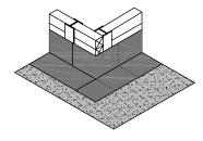
**5.** Embed overlaps into pre-applied HYDRALASTIC 836 and roll press into place.
