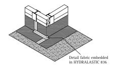
**6.** Apply HYDRALASTIC 836 at all overlapping joints in a 12" wide application and then fully embed detail fabric into this HYDRALASTIC 836. Terminate all edges with additional HYDRALASTIC 836.
