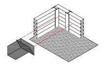
**2.** Cut PRECON on the horizontal to allow for ease of bending around corner.
