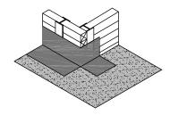
2. Cut PRECON on the horizontal to allow for ease of bending around corner and mechanically fasten according to installation instructions.
