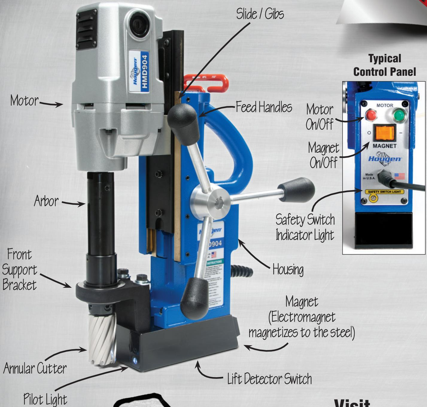
The above drill is the HMD904 which is the most popular drill for general fabrication.
