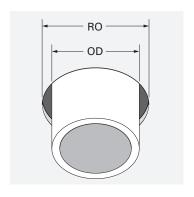
Use **FlexWrap**™ **EZ** only when penetration rough opening (RO) is not more than ½" larger than the outside diameter/ dimension (OD) of non-flanged product.
