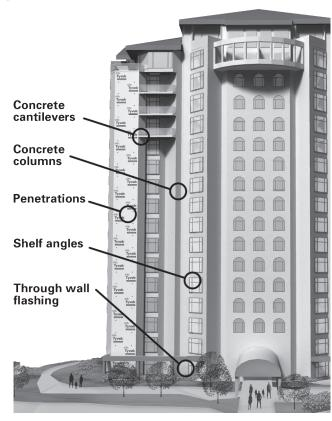
It is important to maintain the continuity of the **DuPont™ Tyvek® WRB** from top to bottom with proper shingling. The entire wall surface shall be wrapped, including unconditioned spaces.
