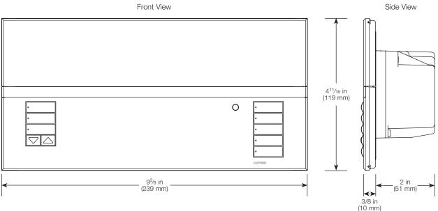
Fits into a 4-gang U.S. backbox, 3<sup>1</sup>/<sub>2</sub> in (90.4 mm) deep (Lutron P/N 245254) or 3 in (76.2 mm) deep (Lutron P/N 241400)
