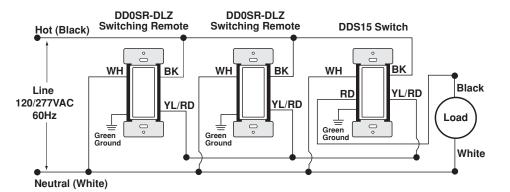
NOTE: The DDMX1 dimmer must be installed in a wall box that has a Load connection. The DD0SR-DLZ dimming remotes NOTE: The DDS15 switch must be installed in a wall box that has a Load connection. The DD0SR-DLZ switching remotes must be installed in a wall box with a Line Hot connection and a Neutral connection
