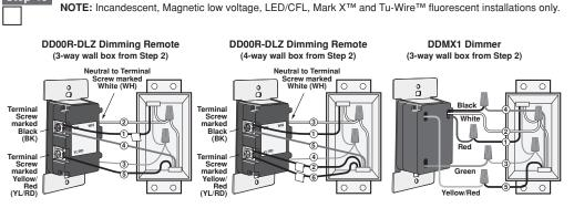
4-Way Wiring - DDMX1 Dimmer with DD00R-DLZ Dimming Remotes Application:
