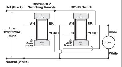
NOTE: The DDS15 switch must be installed in a wall box that has a Load connection. The DD0SR-DLZ switching remote must be installed in a wall box with a Line Hot connection and a Neutral connection
