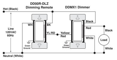
NOTE: The DDMX1 dimmer must be installed in a wall box that has a Load connection. The DD00R-DLZ dimming remote must be installed in a wall box with a Line Hot connection and a Neutral connection
