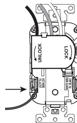
**NOTE:** LOAD wiring terminals accept #10 - #14 AWG solid or stranded copper wire.
