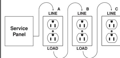
Placing the GFCI in position A will also provide protection to "load side" receptacles B and C. On the other hand, placing the GFCI in position C will not provide protection to receptacles A or B. Remember that receptacles A, B, and C can be in different rooms.
